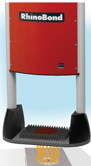
**3** The Flex RhinoBond Induction Tool is placed over the Flex RhinoBond Plate. The tool welds the thermoplastic membrane to the Flex RhinoBond Plate in approximately seven seconds.
