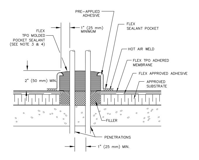
APPLY HEAT TO BASE FLANGE OF FLEX SEALANT POCKET AND FORM BY HAND PRIOR TO HOT AIR WELDING
